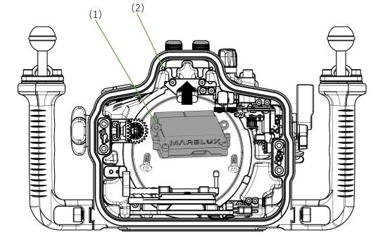
Align the MiniBatt (1) with the screw holes of the housing (2), and then tighten the screws to secure the MiniBatt onto the housing.
