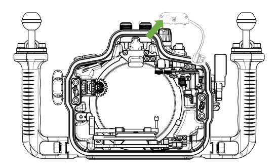
Remove the two screws that secure the Flash Trigger, and then take out the Flash Trigger.
