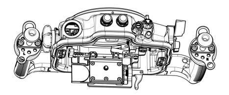
Rotate the cap on the housing counterclockwise to remove it.
