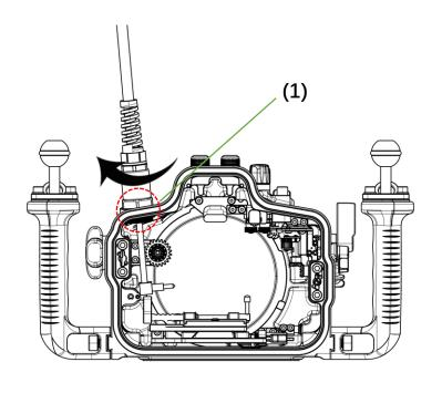
Insert the hydrophone into the M24 port of the housing, and then rotate the component (1) in a clockwise direction as shown in the figure.
