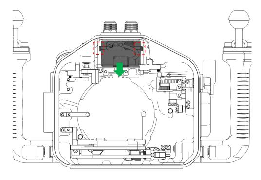
Press and hold the sides of the FlashFuel to remove it (as shown in the picture)
