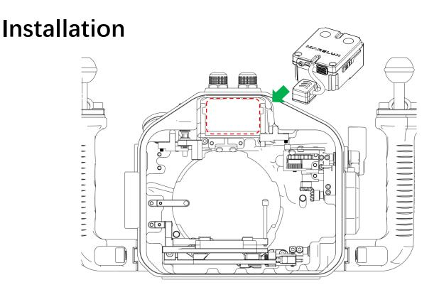
Insert the FlashFuel into the red box area on the housing as shown in the picture.
