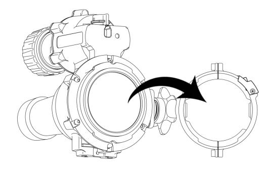
Insert the SOFT as shown in the diagram into the dock, then rotate it clockwise into position.
