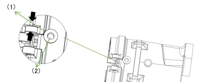
Attach the dock to the strobe so that the notch(1) of the dock aligns to the fiber port(2) of the strobe.
