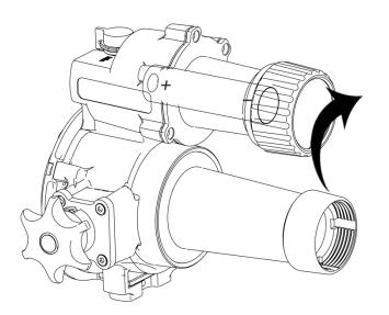
Attach the battery end cap by rotating it clockwise.
