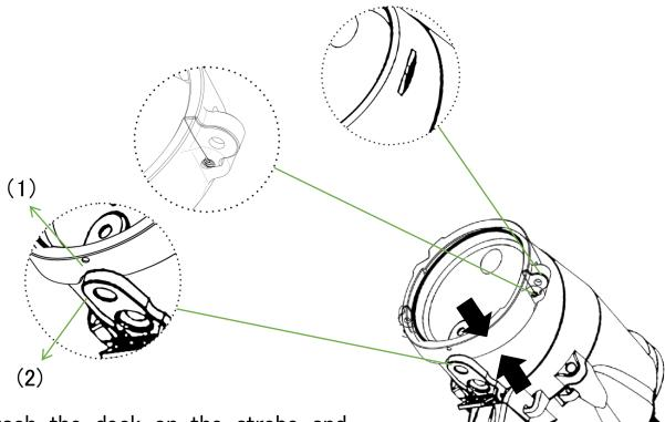
Attach the dock on the strobe and ensure that the notch(1) of dock aligns with the fiber port(2) of strobe.
