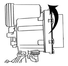
Then attach the dock to the strobe by rotating its ring clockwise.
