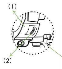
Attach the dock to the strobe so that the notch(1) of the dock aligns to the gear(2) of the strobe.
