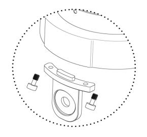
Use screws to attach the mounting ball lock to the dock and tighten them.
