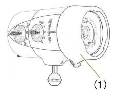
Remove the shroud (1) from the strobe then attach the ring and the dock to the strobe.
