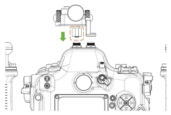
Insert the Lumilink into the camera housing's fiber port.
