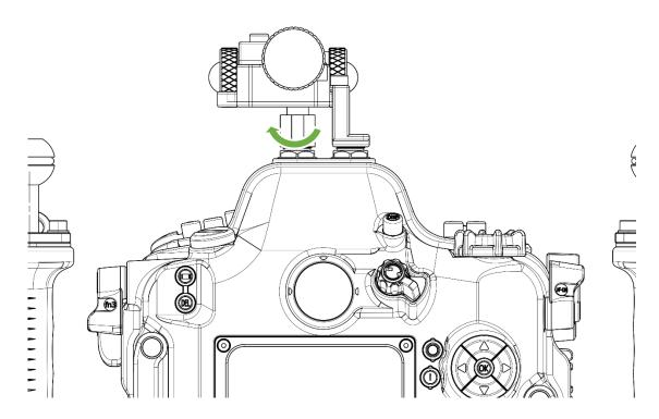
Rotate the bolt clockwise to tighten and secure it.
