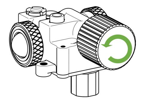
Rotate counter clockwise to remove the battery cap.
