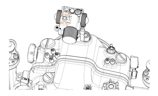
Press and hold the power button for 2 seconds to turn on the Lumilink. The indicator light will stay on continuously. When the shutter button is pressed, it will trigger the Lumilink to emit a blue light signal, triggering the Apollo strobe. There is also a separate fiber optic port on the top, which does not occupy the original fiber optic port of the camera housing.
