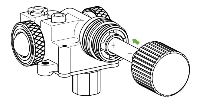
After inserting the battery as shown, rotate clockwise to tighten the battery cap.
